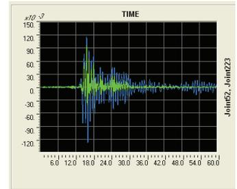
UX displacement, max is  $1.169e-01$  at  $1.564e+01$  (gap 0.02m) - with SSI
