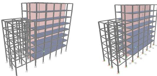
Fig. 3. Two frame buildings, one of them with floors and walls;  $T_1=0.73s$  (xz plane)-without SSI.  $T_1=0.80s$  (xz plane)-with SSI.
