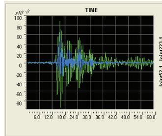
UX displacement, max is  $8.920e-02$  at  $1.558e+01$  (gap 0.02m) - without SSI
